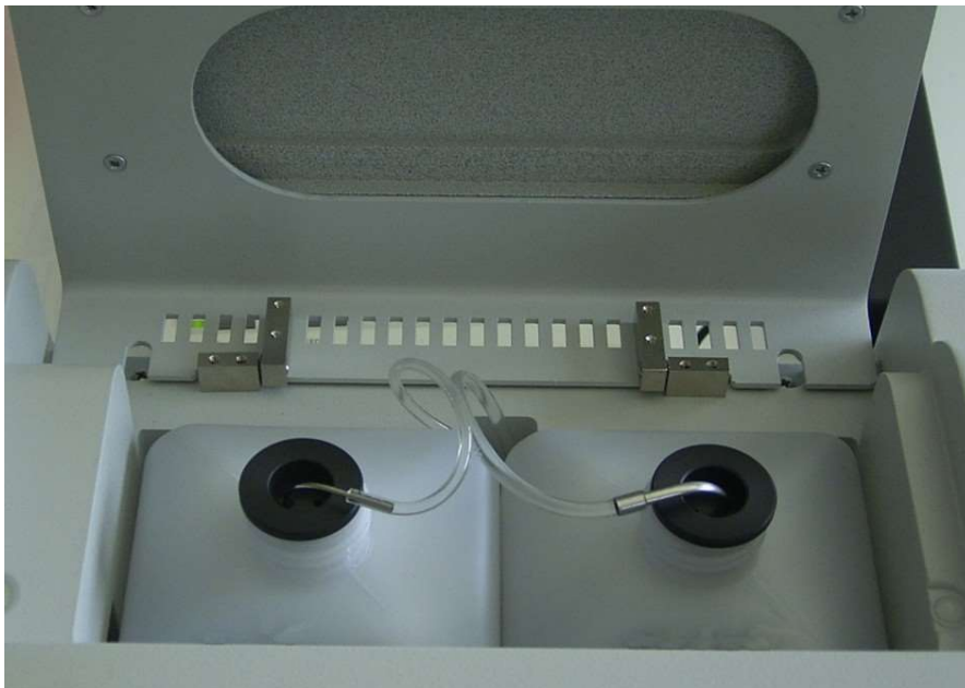
Fig. 6.3 View of supply and waste container
